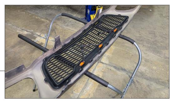
Place the new grille insert into the vehicle grille panel, and press the sides downwards, ensuring the retainers are securing the grille insert. Plug in the wiring harness to each LED light
