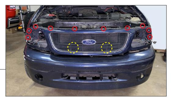
Remove (10) Phillips head screws around the grille. With the screws removed, firmly pull the grille away from the vehicle, noting the (2) central mounting clips. Remove the grille from the vehicle and set on a soft surface for disassembly.
