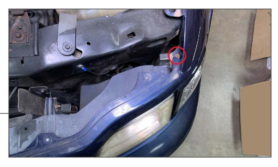
Remove (1) 8mm screw from the inside of the side marker lamp. Unplug the connector and remove the side marker from the vehicle.
