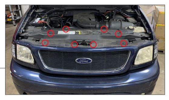
Open the vehicle hood. Remove (8) plastic push clips from the radiator cover. Remove the cover from the vehicle.
