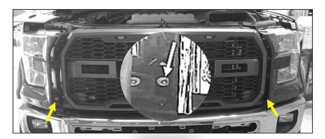
Step 5 Pull back the headlight framing to access the 8mm bolt holding the grille. Remove grille and place onto work table.
