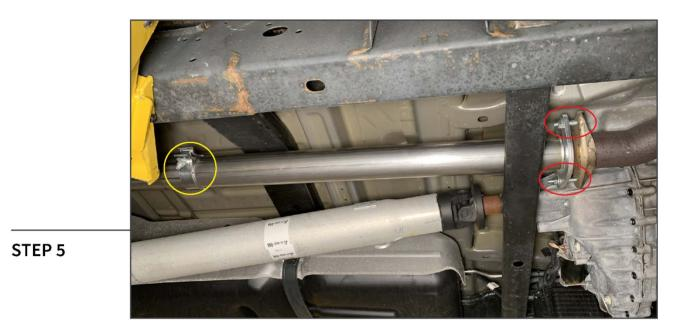
Using (2) M10 bolts, (4) M10 flat washers, and (2) M10 nuts, loosely secure the front pipe to the vehicle exhaust flange.
