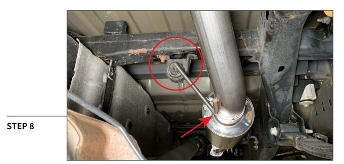
Install the over axle pipe onto the muffler, and loosely secure using (1) previously placed 3" exhaust clamp. Secure the exhaust clamp to the vehicle frame using the original hardware.
