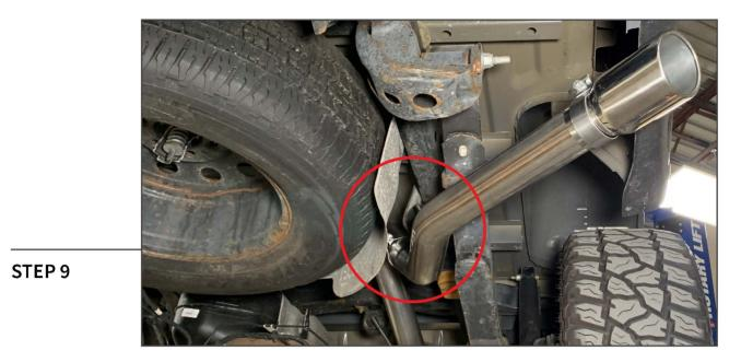
Install the tail pipe pipe onto the over axle pipe, and loosely secure using (1) previously placed 3" exhaust clamp. Secure the exhaust clamp to the vehicle frame using the original hardware.
