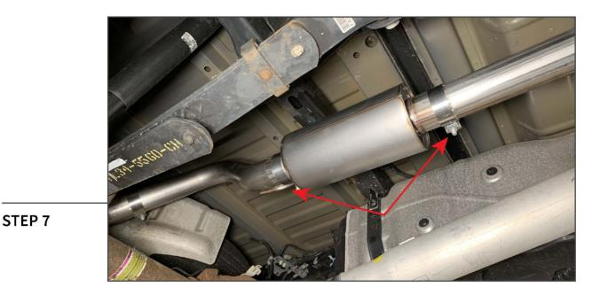
Install the muffler onto the intermediate pipe and loosely secure using (1) previously placed 3" exhaust clamp.
