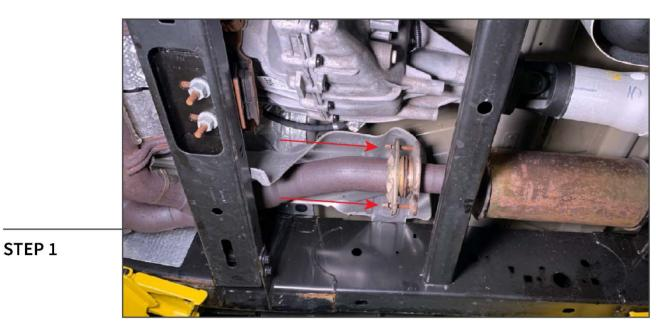
Lift and support the vehicle using a jack and jack stands. Remove (2) 13mm bolts at the front flange next to the vehicle transmission/transfer case.
