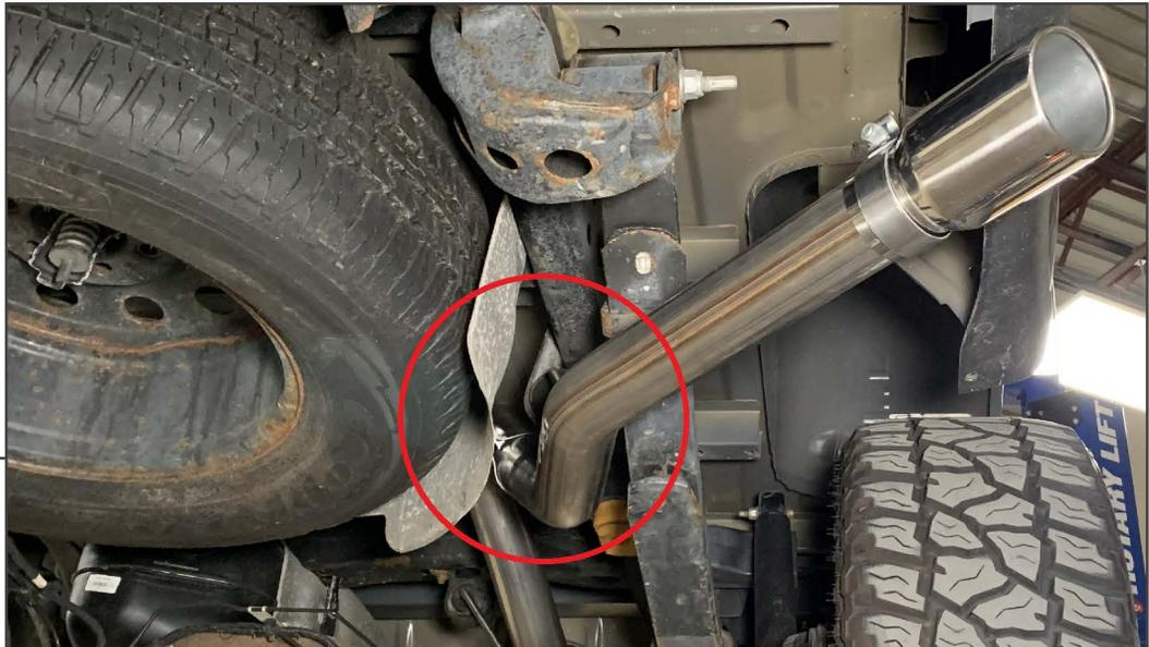
Install the tail pipe pipe onto the over axle pipe, and loosely secure using (1) previously placed 3" exhaust clamp. Secure the exhaust clamp to the vehicle frame using the original hardware.
