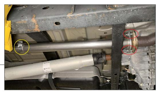
Using (2) M10  $\times$  1.50  $\times$  50mm bolts, (4) M10 flat washers, and (2) M10 nuts, loosely secure the front pipe to the vehicle exhaust flange.
