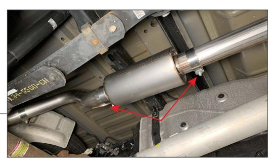
Install the muffler onto the intermediate pipe and loosely secure using (1) previously placed 3" exhaust clamp.
