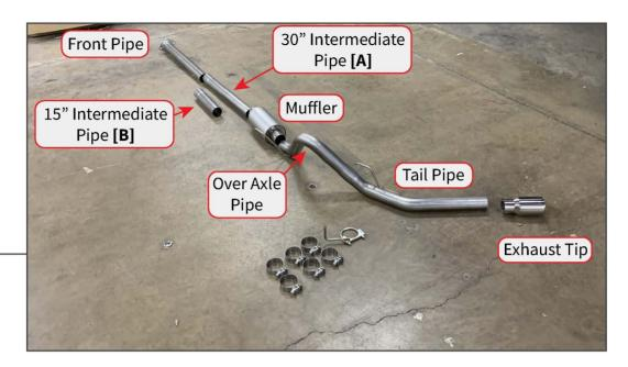
Lay out and identify the different exhaust components. See step 4 regarding intermediate pipes.
