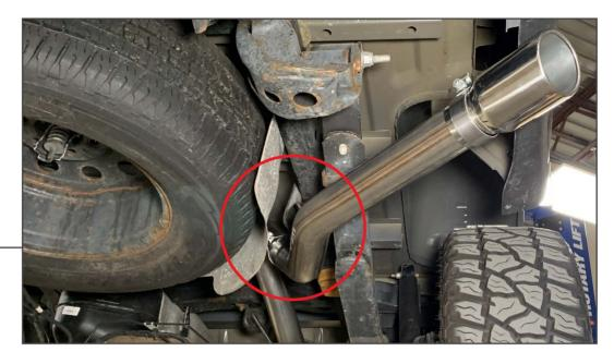
Install the tail pipe pipe onto the over axle pipe, and loosely secure using (1) previously placed 3" exhaust clamp. Secure the exhaust clamp to the vehicle frame using the original hardware.
