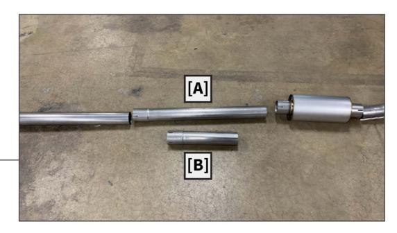
Depending on the vehicle cab/bed configuration, a variation of the intermediate pipes will be used/modified. See the following chart. Wheel Base | Body Style | Bed Length | A | B
