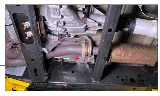
Lift and support the vehicle using a jack and jack stands. Remove (2) 13mm bolts at the front flange next to the vehicle transmission/transfer case.
