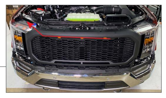
Route the LED wiring harness towards the passenger side headlight assembly. Align the grille assembly to the vehicle and secure the grille to the vehicle re-using original hardware.
