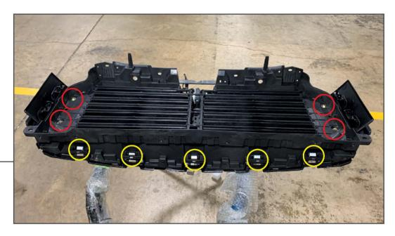
Place the shutter assembly onto the grille ensuring the (5) lower metal clips engage and the (4) shutter mounting studs are through the shutter assembly. Secure the shutter assembly to the grille reusing the original (4) 10mm nuts. Ensure the shutter assembly is seated correctly and not overlapping the wiring harness before tightening hardware. Plug in front emblem wring harness/tube, if applicable.
