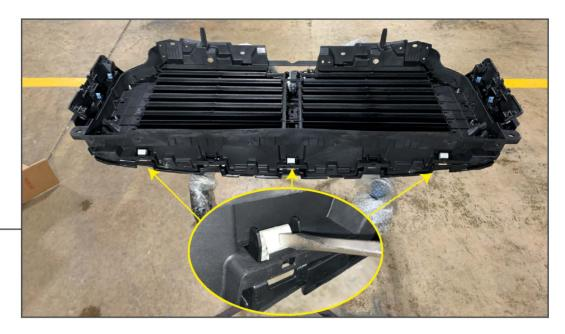
Press in the (3) metal tabs on the grille assembly while lifting upward on the shutter assembly to dislodge the shutter assembly from the grille. Tilt the grille and unplug the front camera/washer assembly hose, if applicable. Remove shutter assembly from the grille. Remove and transfer the (4) shutter mounting studs to the new grille.
