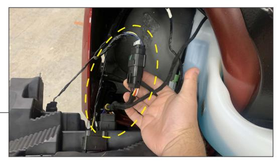
Unplug the main headlight wiring harness. Plug in the 'T' harness into the headlight and the vehicle harness. Neatly route the grille lighting harness to the rear of the headlight and plug the harnesses together.
