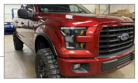
Plug in the (3) original vehicle wiring harnesses to the headlight wiring harnesses, and re-assemble the vehicle with the new headlight following steps 1-12 in reverse order.
