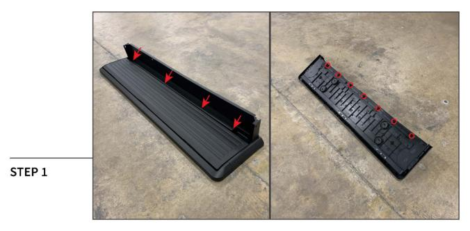
Assemble the vertical panel to the base panel by pressing downwards after aligning the (4) alignment tabs. Then, secure the panels together using (7) Allen head bolts.
