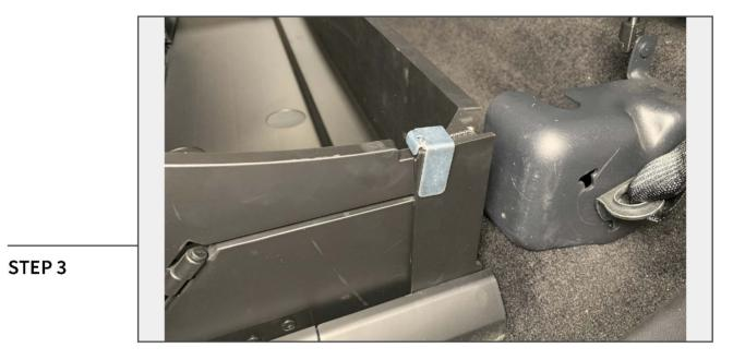
Using the (2) chain brackets, attach the bracket portion to latch the two panels together. Then, route the chain towards the magnet on the vertical panel. This will lock the storage organizer open.
