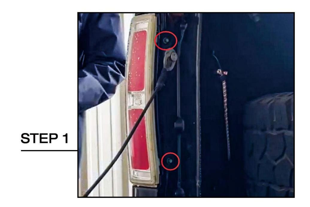
Remove Two 8mm bolts on the top and bottom.
