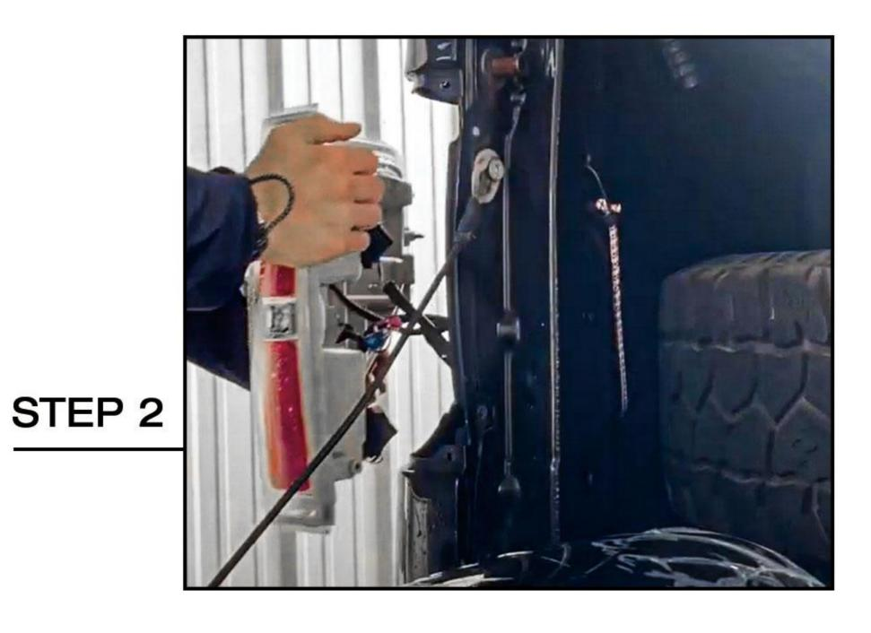
Pull the taillights off the vehicle and unplug the wire harness.
