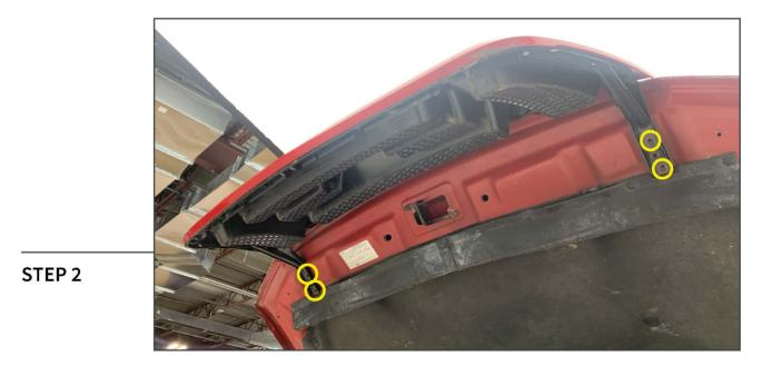
Remove (4) 10mm bolts connecting the grille assembly/brackets to the bottom of the hood. With the hardware removed, gently lower the vehicle hood to remove the grille from the vehicle.
