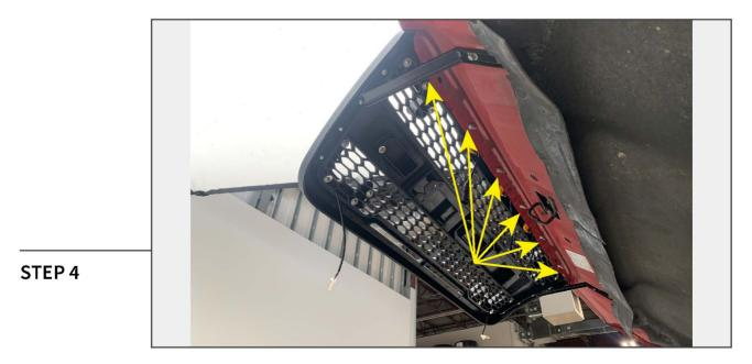
Align the grille to the vehicle, and secure the grille to the front of the hood using (6) M6 flange nuts.
