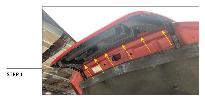
Open the vehicle hood. Remove (6) 10mm nuts connecting the front edge of the hood to the grille.
