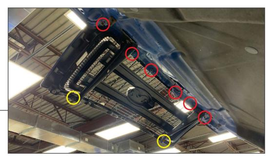
Open the vehicle hood. Locate and remove (6) 10mm nuts and (2) 8mm bolts from the vehicle grille assembly.
