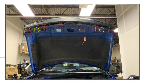
Fit the grille to the vehicle, and secure the top of the grille using the new (6) M6 nuts. Secure the bottom of the grille reusing the original (2) 8mm bolts.
