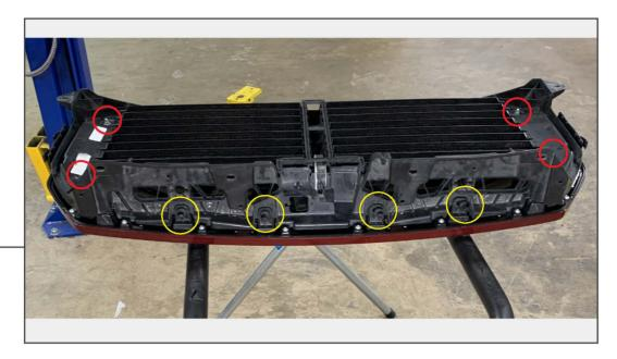
Remove the (4) push clips at the top of the grille, then the (4) 8mm nuts at the bottom. Remove the grille shutter assembly from the grille and transfer it to the new grille.
