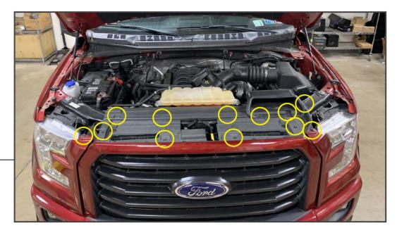
Using a panel removal tool, remove (12) push clips to remove the plastic radiator cover from the grille.
