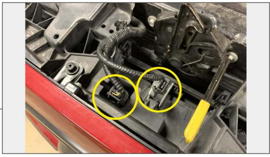
Disconnect the (2) electrical connectors next to the hood latch.
