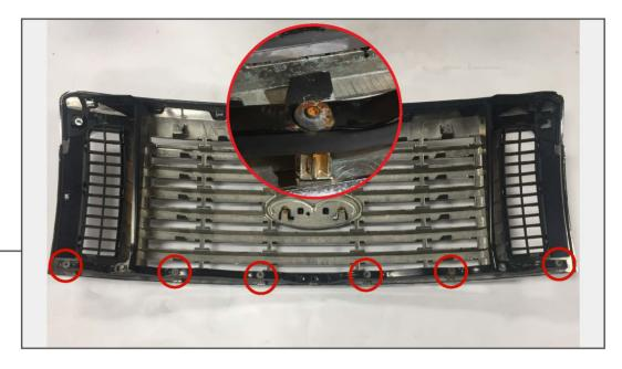
Using a T-25 torx bit, remove the (6) T-25 Torx screws holding the grille brace to the factory grille.
