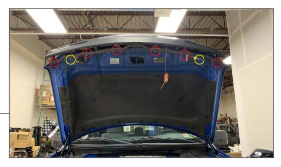
Fit the grille to the vehicle, and secure the top of the grille using the new (6) M6 nuts. Secure the bottom of the grille reusing the original (2) 8mm bolts.
