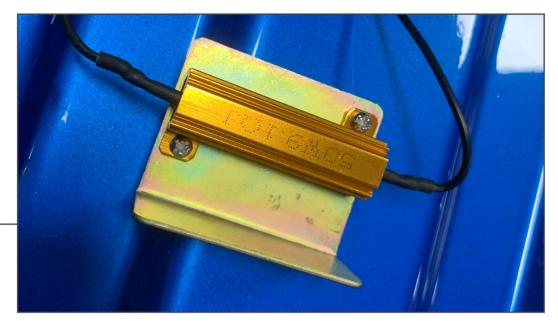
Mount the resistors to the resistor brackets using the supplied hardware. Hold the M4 nut with an adjustable wrench/pliers while tightening the bolts using a Phillips head screwdriver.
