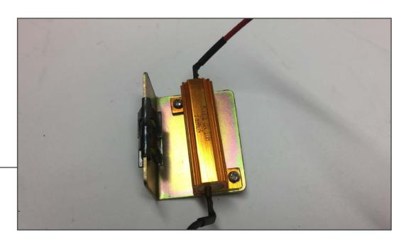
Using (2) vampire clips per bracket, clip each resistor bracket to the vehicle.
