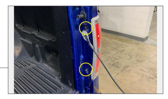
Lower the vehicle tailgate. Remove (2) 8mm bolts from the side of the tail light assembly.
