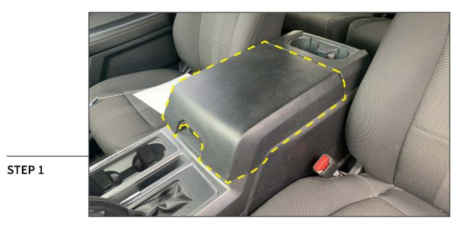
Clean the vehicle center console lid using the provided alcohol prep pads. Once the alcohol is dry, use the adhesion promoter pads over the area the double sided tape will adhere to the console lid, reference the console cover for tape locations.
