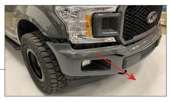
Firmly pull the trim panel away from the vehicle to dislodge the clips. Repeat this procedure to the opposite side. Remove the trim panel from the vehicle and set aside.
