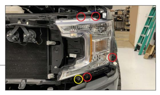
Remove (4) 10mm bolts, and (1) 8mm bolt from the headlight assembly. Remove and unplug the connectors from the headlight assembly. Repeat this procedure to the opposite side.
