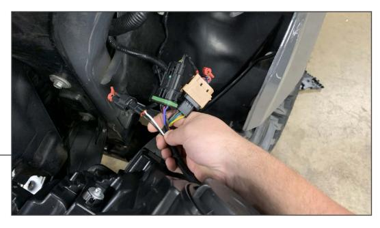
Plug the provided headlight adapter harness into the headlight, and plug in the adapter harness connectors into the vehicle wiring harness. Ensure all connections audibly click into place.
