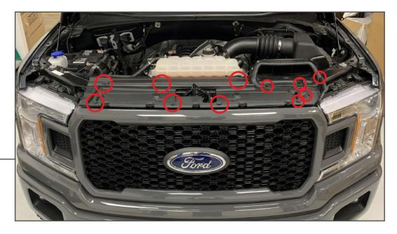
Remove (11) push clips from the upper splash shield. Remove the upper splash shield from the vehicle and set aside.
