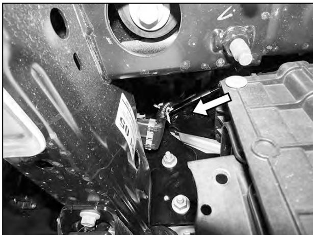
(Fig 3) Unplug all wiring harnesses leading to the front bumper (arrow)
