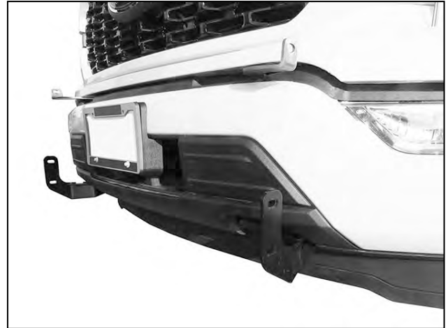
(Fig 14) Brackets installed
