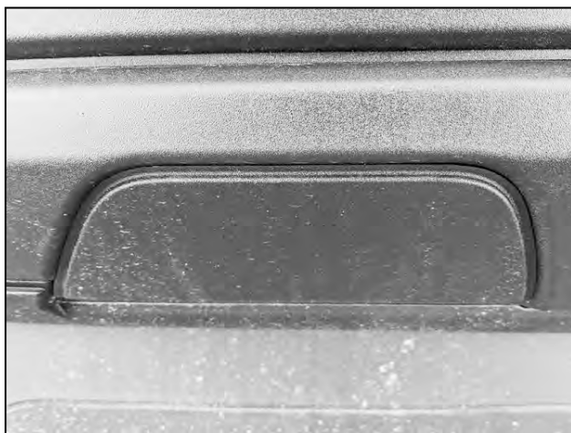
(Fig 10) On models without tow hooks, release clips and remove plastic covers
