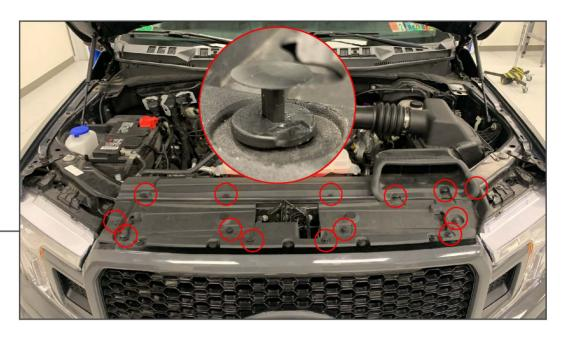
Using a soft pry tool, remove the (14) plastic push pins to remove the air dam from the top of the radiator support.
