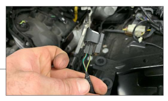
LED Wiring Harness: Using the supplied scotchlok connectors, connect the vehicle parking lamp wiring to the LED light harness using the diagram below. After wiring the LED lights, re-install the headlight using OEM hardware.
