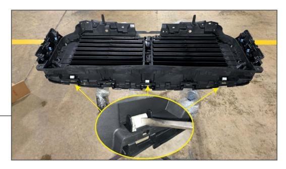
Press in the (3) metal tab clips on the grille assembly while lifting upward on the shutter assembly to dislodge the shutter assembly from the grille. Tilt the grille and unplug the front camera/washer assembly hose, if applicable. Remove shutter assembly from the grille. Remove and transfer the (4) shutter mounting studs and the metal tab clips to the new grille.
