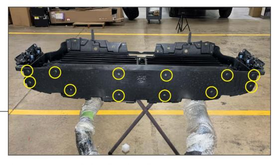
Install the lower splash shield using the (12) original plastic clips.
