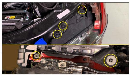
Remove each headlight from the vehicle by removing (2) 10mm upper bolts, (1) plastic clip, (1) lower 8mm bolt, and (1) 10mm nut under the headlight. Firmly pull the light from the vehicle to disengage the (1) mounting stud at the top of the headlight. Splice each LED harness into the vehicle following the diagram using the provided scotchloks.
