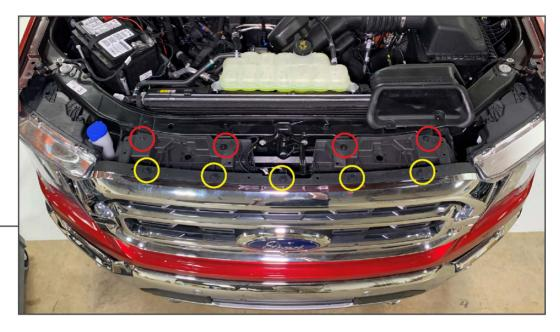
Remove (5) plastic push clips from the top of the grille. Remove (4) 10mm bolts from the radiator support to release the upper portion of the grille.
