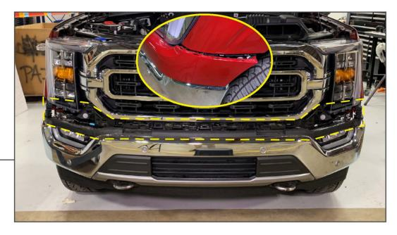
Pull the bumper trim away from the fender by firmly pulling the trim away. Repeat to the opposite side. Firmly pull the bumper trim from the vehicle and set aside.
