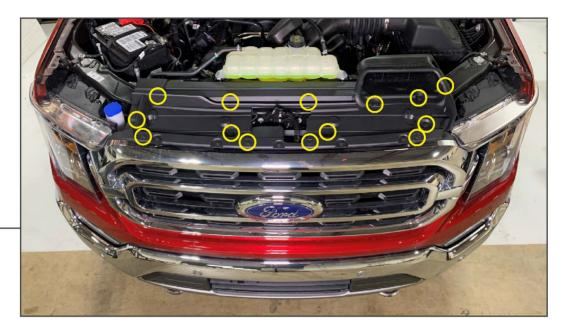
Remove (14) plastic push clips from the radiator cover. Remove radiator cover and set aside.
