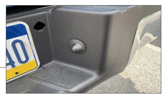
Fit the new housing onto the vehicle license plate lamp socket, and twist the socket clockwise to secure the socket into the housing. Press the light socket into the vehicle until the mounting tabs audibly click into place.
