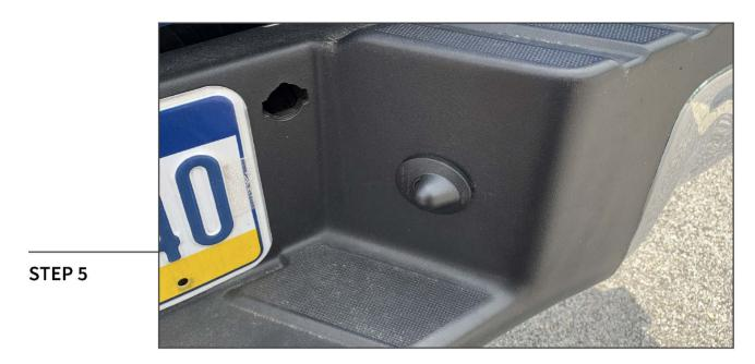
Press the light socket into the vehicle until the mounting tabs audibly click into place.
