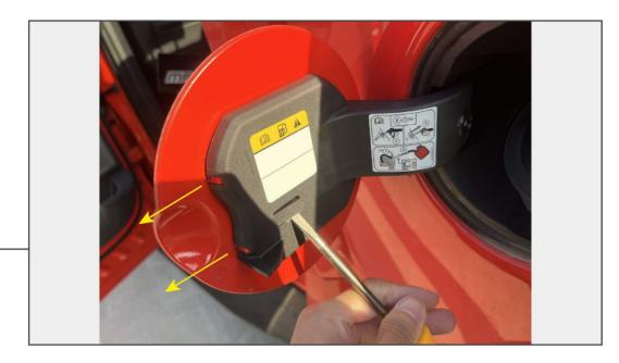
Using a flathead screwdriver, lift the plastic retaining tab on the fuel door. With the retaining tab lifted, slide the fuel door away from the vehicle.
