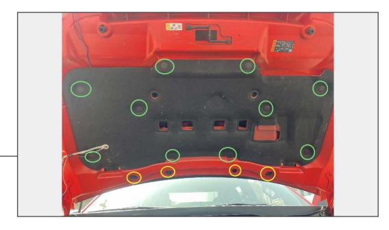
Open the vehicle hood. Remove (10) plastic pins from the hood insulation, and (4) plastic caps from the hood.
