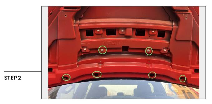
Remove (6) 10mm nuts from the under-side of the hood.
