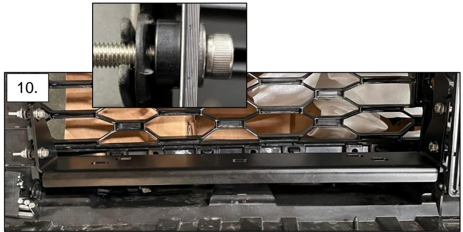
11. Using a 7/16" socket, attach the bracket to the lightbar.
