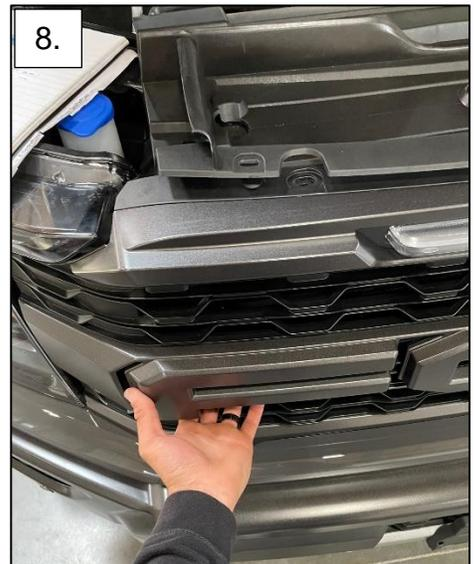
9. Using a flat head screwdriver remove the required amount of lower plastic shutters by bending the plastic tab away from the shutter releasing the pivot pin. They will need to be removed on each side. Onx6 kits will need the 4 lower shutters removed. S8 Kits will need the 3 lower shutters removed.
