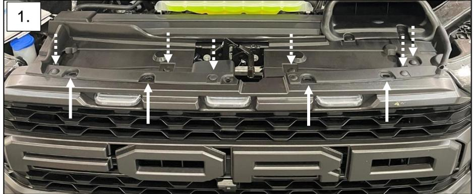
2. Fold up the rubber radiator shroud and disconnect all the electrical for the front grille. There will be a total of 4 connectors (↗) and 2 plastic rivet push clips (↖).
