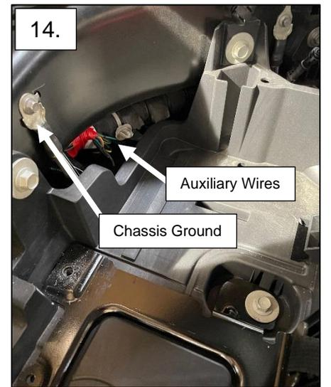
15. **S8 Kit Only:** Separate the auxiliary wires. Use either auxiliary wire 2 (Green/Brown) or 3 (Green/Blue) for the main power (White Wire). Take the clasp connector on the up-fitter harness and close over the desired wire using pliers. If the backlighting feature is desired, take the clasp connector on the additional green wire, and close over any auxiliary wire.
