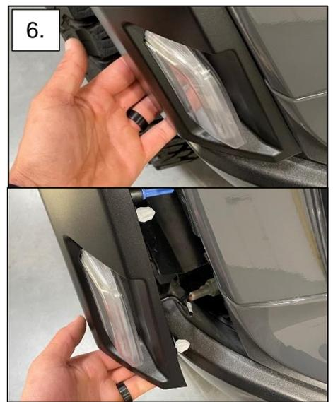
7. Pull on the front grille fascia to remove from the front fender. Repeat process on both sides.
