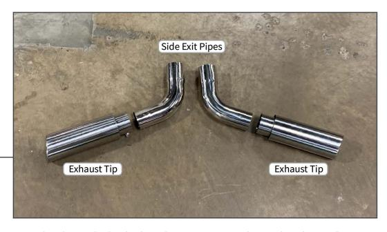
If the vehicle is equipped with a trailer hitch, the side exit pipes must be used as shown above.
