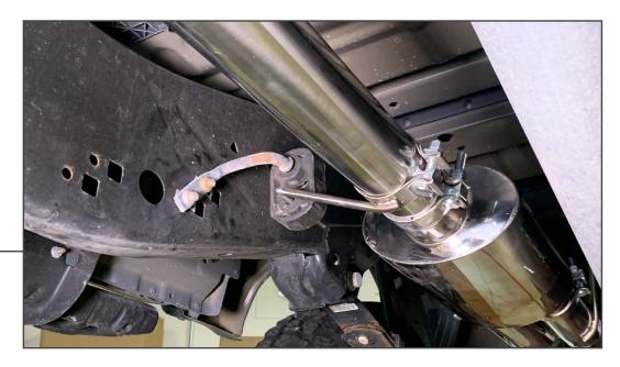
If required, slide the mid pipe onto the front pipe with an exhaust clamp. Then, install the clamp hanger so that it aligns with the factory frame mounted exhaust hanger right before the muffler. Reuse the factory rubber isolator and bolts.
