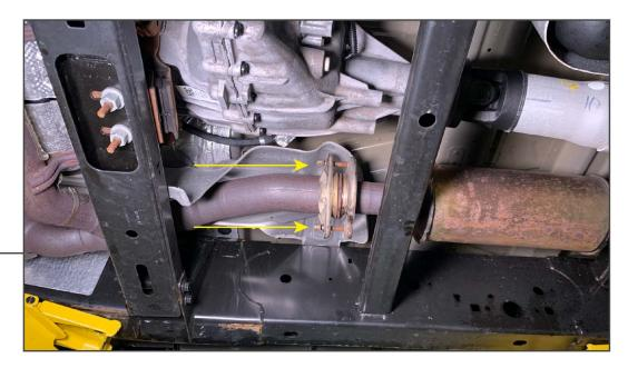
Begin by raising and supporting the vehicle to gain better access to the factory exhaust system. Locate the factory (2) bolt exhaust flange located to the right of the transmission/transfer case. Use a 13mm socket to remove the factory bolts. \*\*Note: Factory hardware will not be reused.
