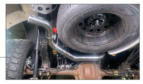
Hang the left side exhaust pipe using the provided isolator and hanger installed in step 3.
