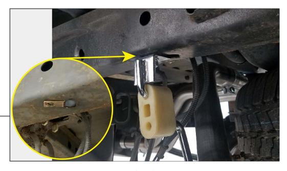
Install the supplied exhaust hanger on the driver side of the frame. Insert the supplied clip nut on the driver side of the frame rail from the square hole into the round hole. Then, install the supplied exhaust hanger using the provided (1) M8 x 30mm bolt, flat washer, lock washer. Torque to 18ft.lbs.
