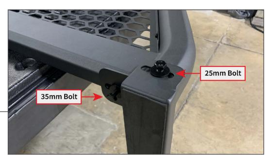
Loosely secure the bed mounting brackets to the headache rack using (1) M10 x 35mm bolt, (1) M10 x 25mm bolt, (2) M10 lock washers, and (2) M10 flat washers per bracket. The mounting brackets must be loose to allow for adjustments later.
