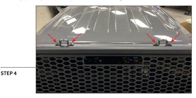
Secure the (2) light bar raising brackets to the headache rack using (2) M8 x 25mm Allen bolts, (2) M8 lock washers, and (2) M8 flat washers per bracket into the headache rack threaded inserts. Pod lights can be installed to these mounting brackets. See step 5 for light bar mounting.
