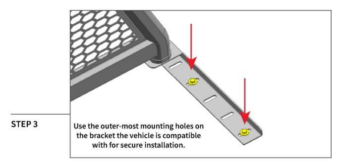
Use a permanent marker to mark the vehicle bed rail for drilling, then remove the headache rack from the vehicle. Drill (2) holes in the bed rail to fit the M10 hardware using a 13/32" drill bit. Once drilled, secure each side of the headache rack to the vehicle bed using (2) M10 x 50mm bolts, (2) M10 lock washers, (4) M10 flat washers, and (2) M10 nuts. Tighten evenly until secure.
