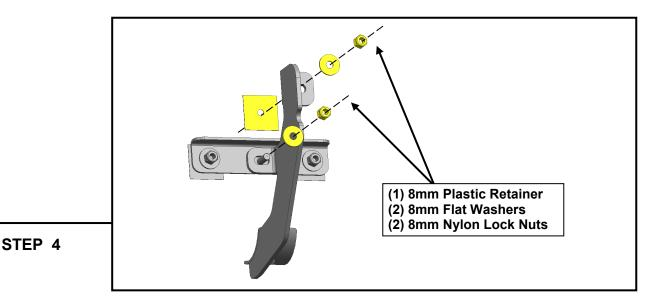
Loosely attach the (1) Passenger step bracket to the upper factory mounting stud and the (1) Passenger reinforcement bracket using (1) M8 plastic washer, (2) M8 flat washers, and (2) M8 nylon lock nuts.
