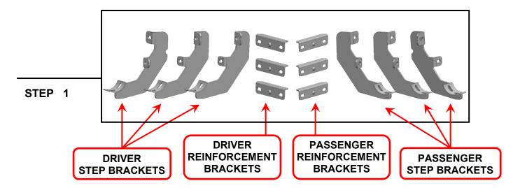
Identify each mounting bracket using the engraved location identifier. Notice: The Center brackets are the same as The Rear brackets. Both Reinforcement brackets are the same.
