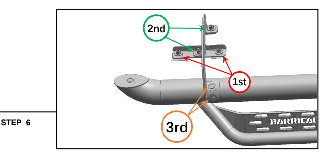
Tighten the mounting brackets to the vehicle. Adjust the side step to the desired angle, and tighten the M8 combo bolts to secure the step into place. See photo for tightening order visual.
