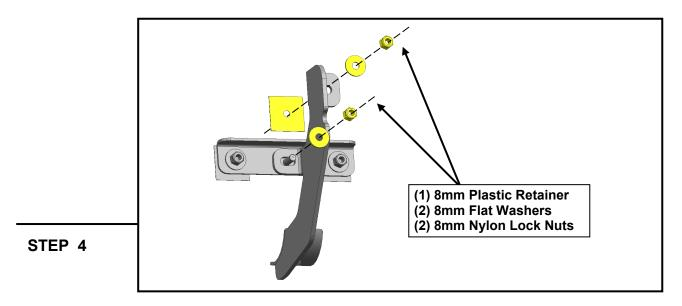
Loosely attach the (1) Passenger step bracket to the upper factory mounting stud and the (1) Passenger reinforcement bracket using (1) M8 plastic washer, (2) M8 flat washers, and (2) M8 nylon lock nuts.
