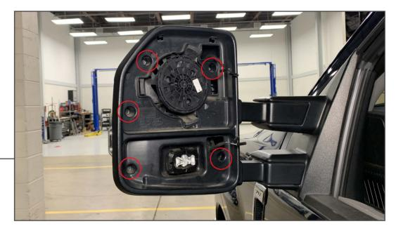
Remove (5) 7mm screws from the mirror housing.
