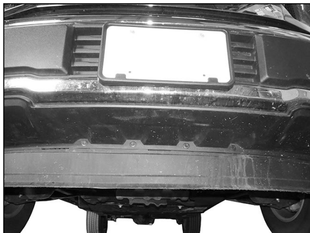
(Fig 1) Remove license plate from Bumper
