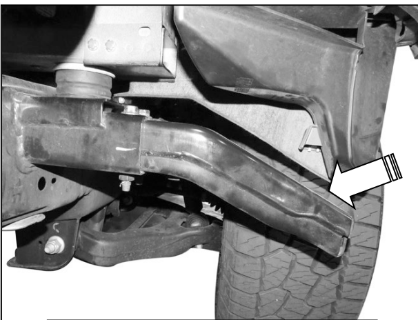
(Fig 8) Optional, remove the factory frame extensions, if equipped
