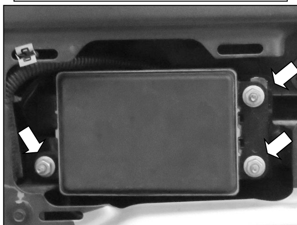
(Fig 3) Unplug and remove adaptive cruise control sensor from driver/left side of frame, if equipped
