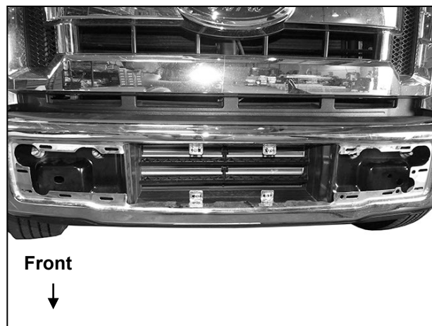
(Fig 2) Remove the plastic bumper pad from the front of the Bumper
