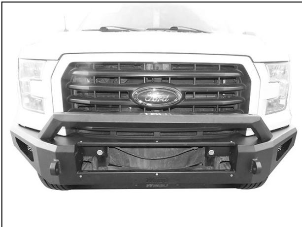
(Fig 12) Center and align the Bumper to the vehicle and fully tighten all mounting hardware. (Hoop pictured not included)
