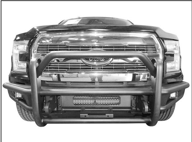
(Fig 8) Push Bar installed (without U-Covers). Note lights pictured not included
