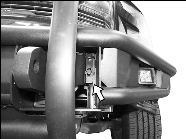
(Fig 7) Reuse the outer Double Bolt Plate to attach the driver/left side of the Push Bar to the PB Shackle Bracket and Bumper
