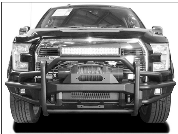
(Fig 10) Attach driver/left "L" Bracket to tab on back of Push Bar
