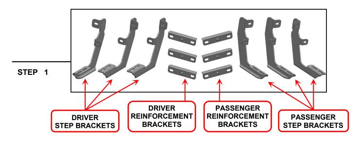
Mounting Brackets look very similar but are unique. Please identify each mounting bracket using the engraved location identifier. Notice: The Center brackets are the same as The Rear brackets. Both Reinforcement brackets are the same.
