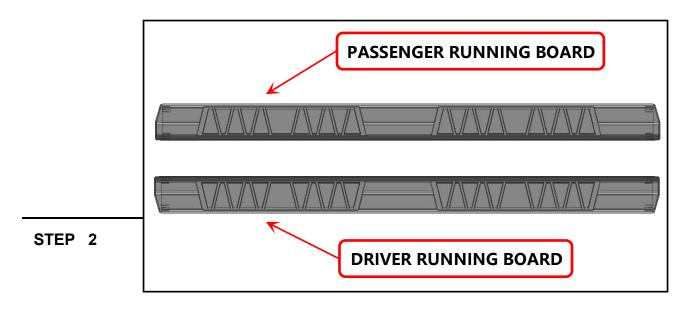
Identify each side step by the front of the step. Notice: The Passenger/Right Running Board will have a "P" on the front.
