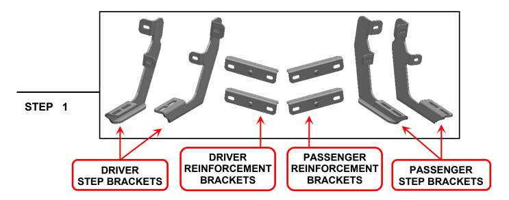
Mounting Brackets look very similar but are unique. Please identify each mounting bracket using the engraved location identifier. Notice: Both Reinforcement brackets are the same.
