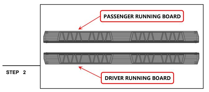
Identify each side step by the front of the running board. Notice: "D" for Driver/Left Side; "P" for Passenger/Right Side.
