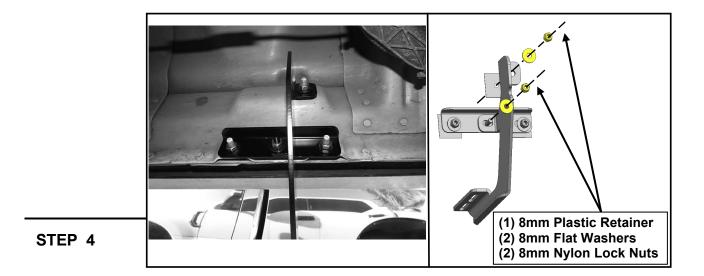
Loosely attach the (1) Passenger step bracket to the upper factory mounting stud and the (1) Passenger reinforcement bracket using (1) M8 plastic washer, (2) M8 flat washers, and (2) M8 nylon lock nuts.
