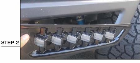
Press fog lights directly into the opening of the front bumper firmly. The lights have four brackets in the back (2 top, 2 bottom) and they snap onto the edges of the openings.
