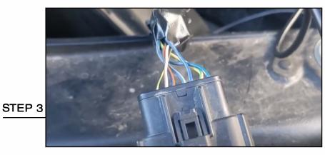
Identify the wire harness that comes out of the back of the driver's side headlight: the wire all the way to the right is going to be your directional for the driver's side; the third wire from the right is going to be your DRLs; the brown wire is going to be your headlight; the black and yellow wire is the ground in the harness. Use the included scotchlok connectors to splice onto those wires, and install and hook up the lights.
