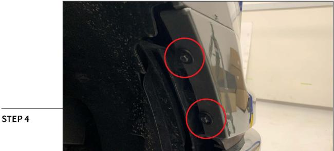
Remove (2) 7mm bolts from inside the fender well.
