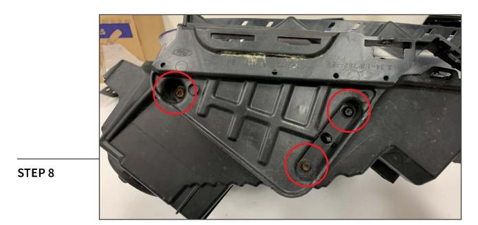
Remove the lower headlight mount from the headlight assembly by removing (3) T-25 Torx screws. Transfer the lower headlight mount to the new headlight assembly reusing the original T-25 Torx screws.
