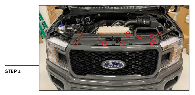
Remove (11) push clips from the upper grille cover. Remove the cover from vehicle.
