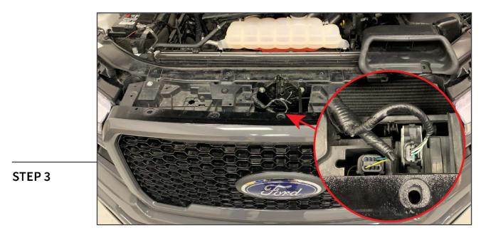
Unplug the (2) electrical connectors from the top of the grille by pushing in the plastic tab on each connector.
