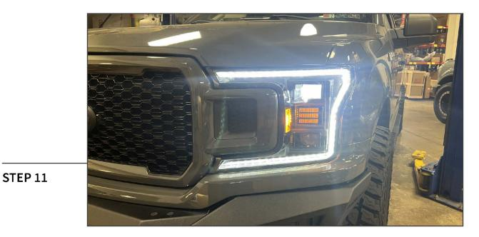
Fit the new headlights into the vehicle, and secure each headlight using the OEM headlight mounting hardware on each side of the vehicle.
