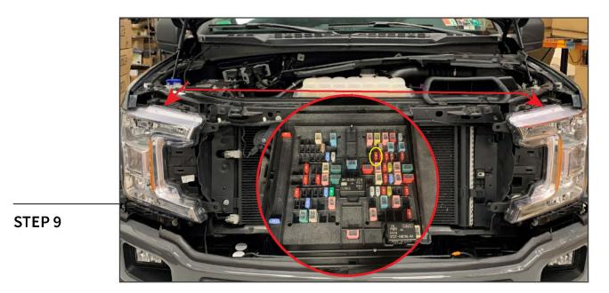
Route the provided DRL wiring harness neatly from the fuse box, across the engine bay to both headlight assemblies. Replace the indicated fuse with the DRL harness. Secure the DRL harness from any hot/moving components using cable ties.
