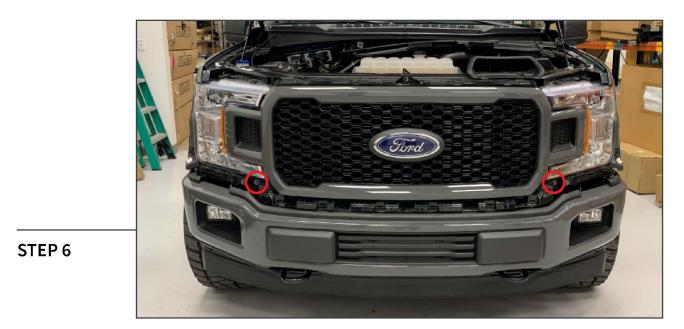
Remove (2) 8mm bolts from the bottom of the grille assembly. Remove the grille assembly from the vehicle.
