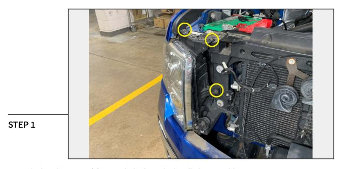
Open the hood. Remove (3) 10mm bolts from the headlight assembly.
