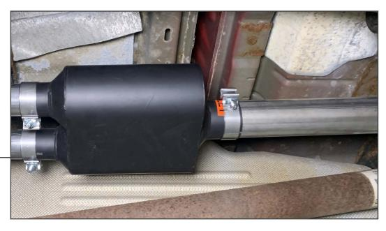
Fit the muffler to the front/intermediate pipe, and loosely secure using the previously placed 3" exhaust clamp.
