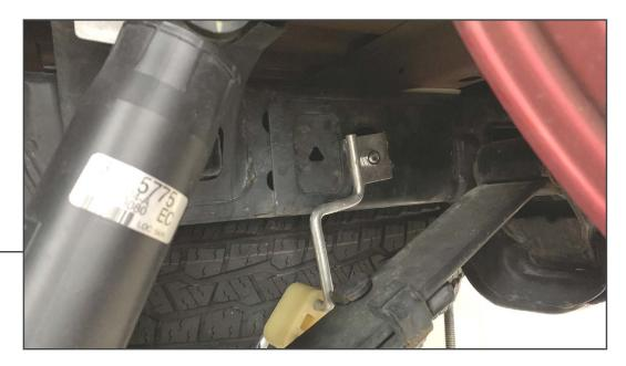
Locate the holes along the LH side frame rail. Fit the (1) hanger bolt with (1) flat washer through the round frame hole with a magnet tool. Then, fit the hanger bracket into place. Secure the hanger bracket into place using (1) flat washer, (1) lock washer, and (1) nut. Tighten until secure.
