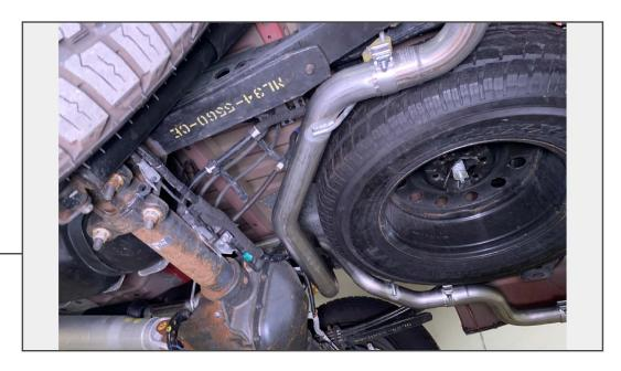
Fit the LH exit pipe into the LH over-axle pipe, then fit the pipe hanger into the previously placed rubber hanger along the frame. Loosely secure the pipes together using the previously placed exhaust clamp. Use the included zip tie to relocate the differential sensor wires/line if necessary.
