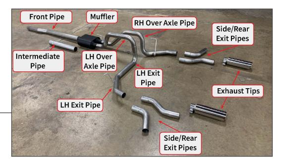
Lay out and identify the included exhaust components.
