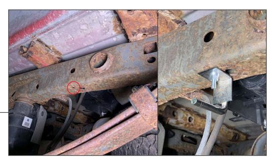
Locate the holes along the LH side frame rail. Fit the (1) 5/16 bolt with (1) flat washer through the round frame hole with a magnet tool. Then, fit the hanger bracket into place. Secure the hanger bracket into place using (1) flat washer, (1) lock washer, and (1) nut. Tighten until secure.
