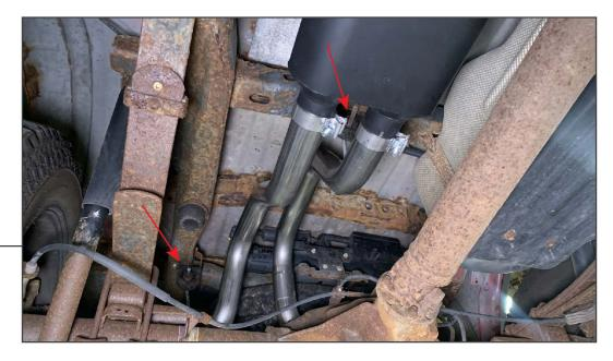
Fit the LH and RH over-axle pipes into the muffler, and fit each pipe into the vehicle rubber hangers in the vehicle frame. Loosely secure the pipes to the muffler using the previously placed clamps.
