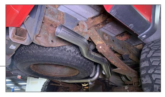
Fit the desired exit pipe to the exhaust system, and loosely secure using the previously placed exhaust clamp.
