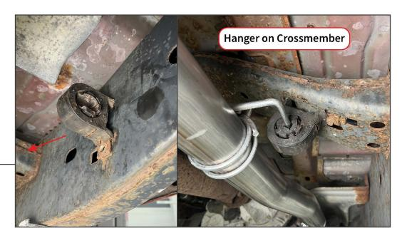
Fit the included hanger clamp to the front pipe. If necessary, relocate the OEM rubber exhaust hanger from the side of the frame to the crossmember above the front pipe using the OEM hardware. Then, fit the hanger clamp into the hanger and tighten into place.
