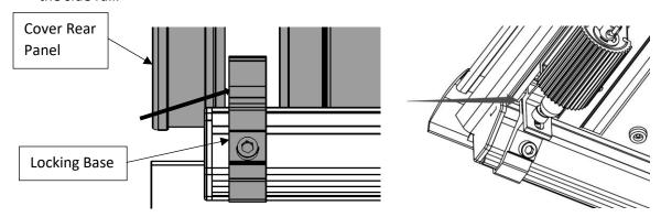
13. If the locking pin on the cover interfere with the locking tongue on the locking base, adjust the locking tongue up and down to a proper position, then tighten the bolt to fix the locking tongue.
