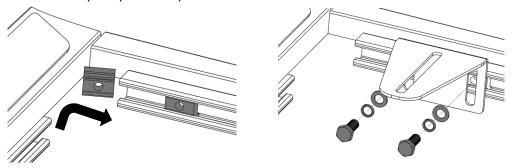
For 2024 Ford Ranger, Attach the bracket (F15) to the threaded hole in the front bulkhead of the truck bed.
