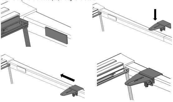
7. Stick the foam seal tape (F10) on the front edge of the bed. The tape length is same as the bed front inner width. Cut off the extra foam.
