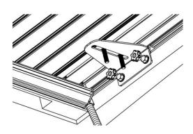
11. Insert the Security Straps (F5) onto the Front Bolt firstly, then insert Flat Washer (F7), Spring Washer (F8), and T Type Nut (F9). Tighten the T type nut firmly.
