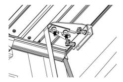
12. Close the cover, adjust the locking base back-and-forth to accommodate the groove of the rear panel. Try to close and open the cover rear panel several times. Make sure the Locking Base does not interfere with the groove of cover rear panel. Then tighten the bolt to fix the locking base on the side rail.
