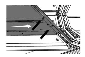
10. Close the cover front panel, and insert the Front Bolts (F6) into the bolt hole of the front bracket.
