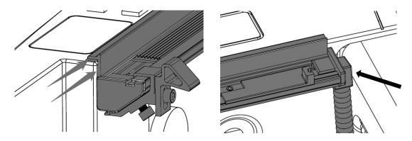
5. Place one clamp A (F11) at the front of the side rail and one at the rear (please make sure the rear clamps is placed on the position that is closest to tailgate). Tighten the clamps each side. Then insert the drain tubes (F4) into the front of bed wall.
