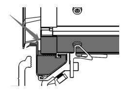
9. Roll up the cover front panel, making the back of front panel facing up. Insert the Front Bolt (F6) into the grooves of the front panel.
