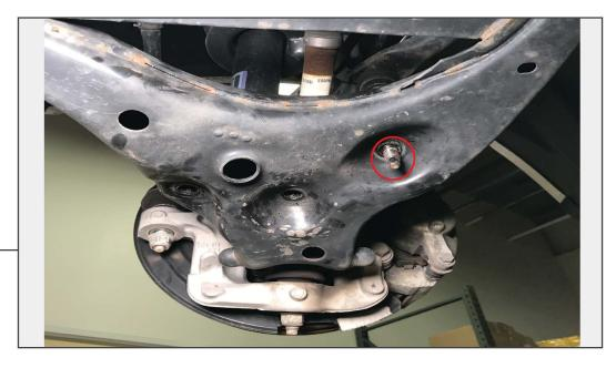
Using a 18mm socket, remove the nut from the sway bar end link.
