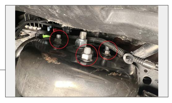
Visualize the coilover strut upper studs. Lift and align the studs with the holes in the vehicle frame. If the holes do not initally align, spin the strut until all three studs fit into the frame. Loosely secure the coilover strut using the included (3) flange nuts.
