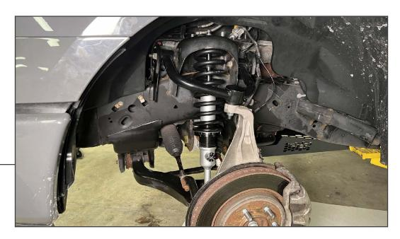
Re-assemble the vehicle front suspension following 1-6 in reverse order. See last page for dampening adjustments.
