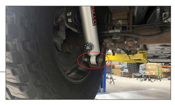
Fit the new shock absorber to the vehicle axle mount using the original shock bolt.
