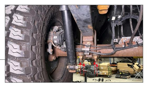
With the jack supporting the vehicle axle, loosen the (4) 21mm leaf spring U-Bolt nuts. Loosen the bolts evenly until the nuts are completely removed.
