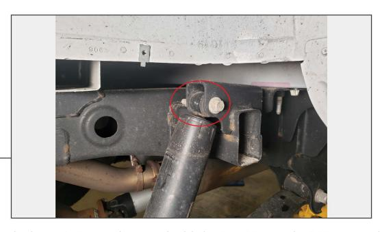
Locate the upper shock mount. Remove the upper shock bolt using a 15mm socket & 18mm wrench.
