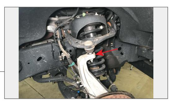
Using a 18mm socket, loosen the nut securing the upper ball joint to the knuckle. Using a sledge hammer, strike the knuckle to separate the ball joint from the knuckle. Remove the nut to separate the control arm from the knuckle.
