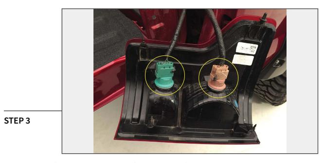
Disconnect the factory tail light harness from the back of the bulb housing.
