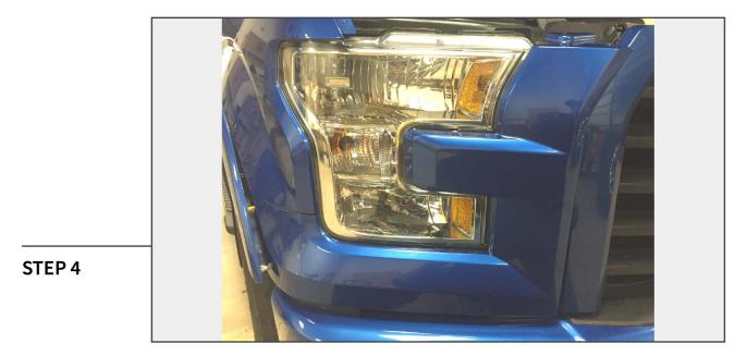
Carefully pry the headlight cover from the headlight assembly to dislodge the retaining clips. Set the cover aside.
