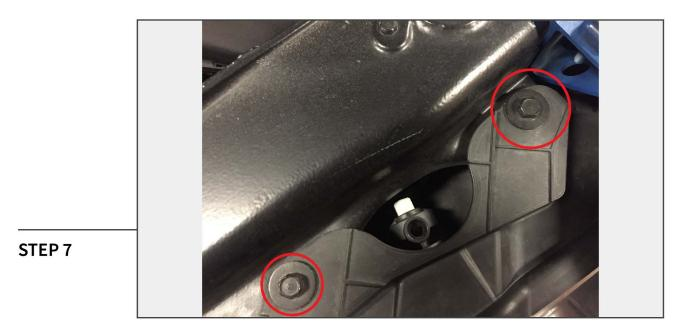
Remove (2) 10mm bolts from the top of the headlight assembly.
