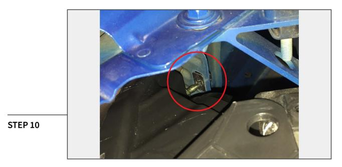
Carefully pry the headlight from the locating retainer.
