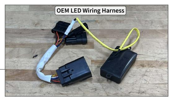
Determine the required wiring harness for the vehicle. The pre-installed harness is OEM Halogen headlights. If the vehicle has OEM LED headlights, remove the pre-installed harness and install the OEM LED harness.
