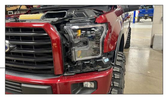
Plug all headlight harness connectors into the vehicle wiring harness. Plug the DRL harness into the (1) DRL harness connector [blue wire].
