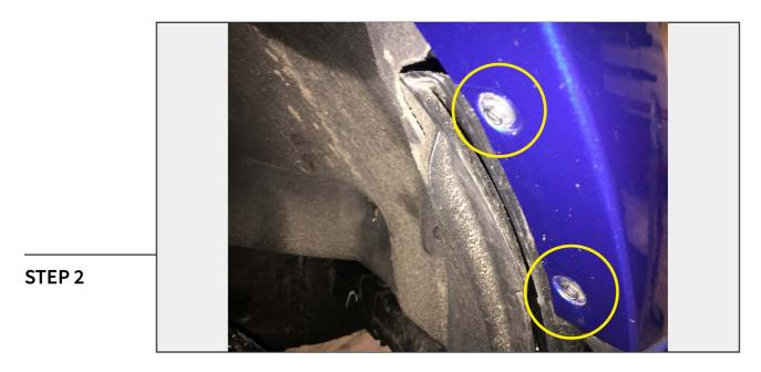
Remove (2) 7mm screws from the inner fender liner/flare.
