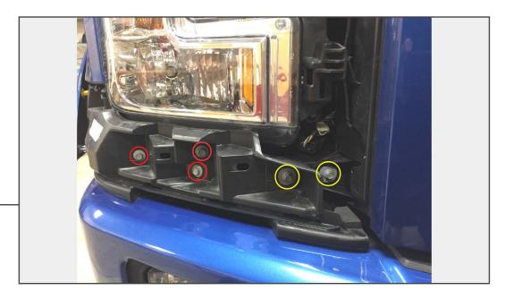
Remove (3) 10mm bolts and (2) 8mm bolts from the lower portion of the headlight assembly.
