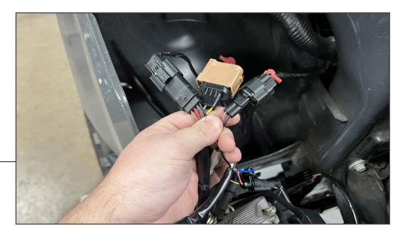
Plug each headlight harness into the appropriate vehicle wiring harness. Plug the DRL harness into each headlight DRL harness.
