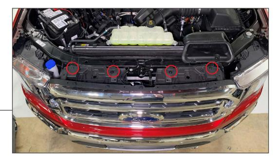
Remove (4) 10mm bolts from the radiator support to release the upper portion of the grille.
