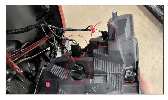
Unplug the wiring harnesses from the vehicle headlight assembly.
