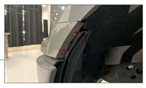
Remove (2) 7mm screws on each side of the vehicle securing the front fascia to the vehicle.
