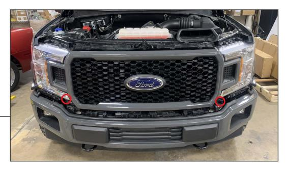
Remove (2) 13mm bolts along the bottom of the grille. With the bolts removed, pull the front grille assembly from the vehicle. Place the grille on a soft workable surface.
