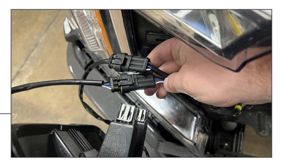
Re-install the headlight to the vehicle using the OEM hardware, ensuring to route the grille lighting leads neatly out of the headlight mounting area.
