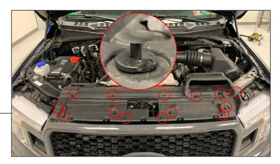
Using a soft pry tool, remove the (14) plastic push pins to remove the air dam from the top of the radiator support.
