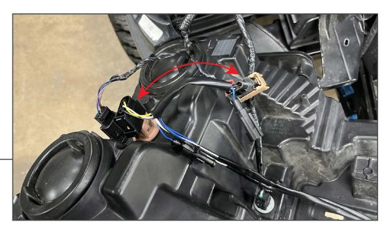
Plug the (1) 'T' harness into the appropriate headlight connectors and the vehicle harness.
