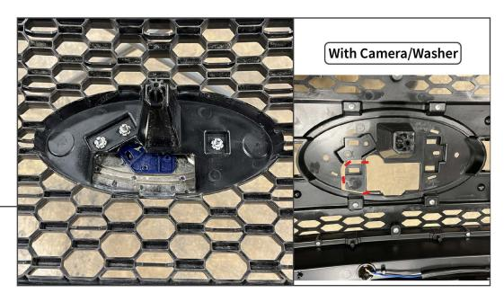
Remove the grille emblem from the grille by removing the (3) nuts. Transfer the emblem to the new grille reusing the (3) nuts.
