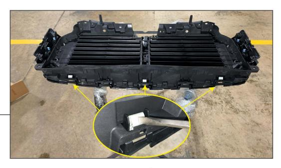
Press in the (3) metal tab clips on the grille assembly while lifting upward on the shutter assembly to dislodge the shutter assembly from the grille. Tilt the grille and unplug the front camera/washer assembly hose, if applicable. Remove shutter assembly from the grille.
