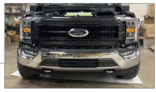
Fit the grille to the vehicle, and plug in the grille lighting connectors into the 'T' harness.
