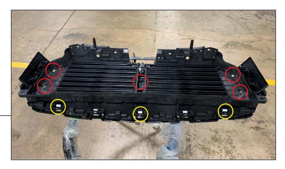
Verify the grille lighting harnesses are routed to the top of the grille. Then, place the vehicle shutter assembly onto the new grille, and engage the pre-installed lower metal tab clips. Secure the shutter assembly into place using the original (4) 10mm nuts and (1) 8mm screw, tighten hardware evenly until secure.
