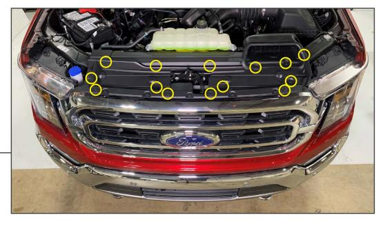
Remove (14) plastic push clips from the radiator cover. Remove radiator cover and set aside.
