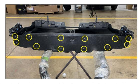
Remove (12) plastic clips from the lower portion of the grille. Remove the (4) plastic clips from each side splash shield. Remove the splash shields and set aside.
