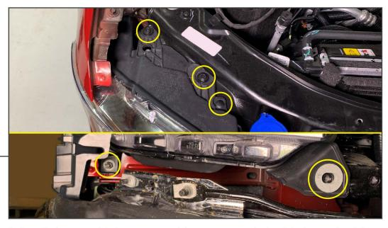
Remove the RH side headlight assembly by removing (2) 10mm upper bolts, (1) plastic clip, (1) lower 8mm bolt, and (1) 10mm nut under the headlight.
