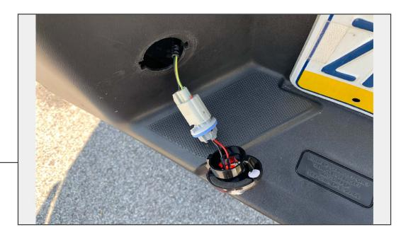
Plug the LED license plate lamp into the vehicle.
