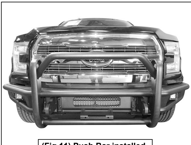
(Fig 11) Push Bar installed (without U-Covers)
