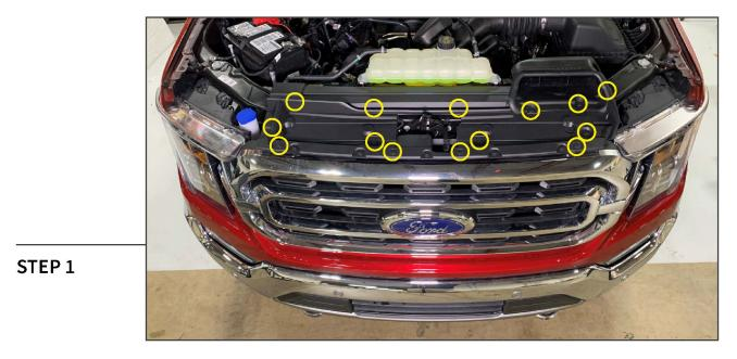
Remove (14) plastic push clips from the radiator cover. Remove radiator cover and set aside.
