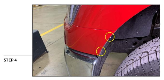
Remove (2) 7mm bolts from inside the fender well. Repeat this procedure to the opposite side.
