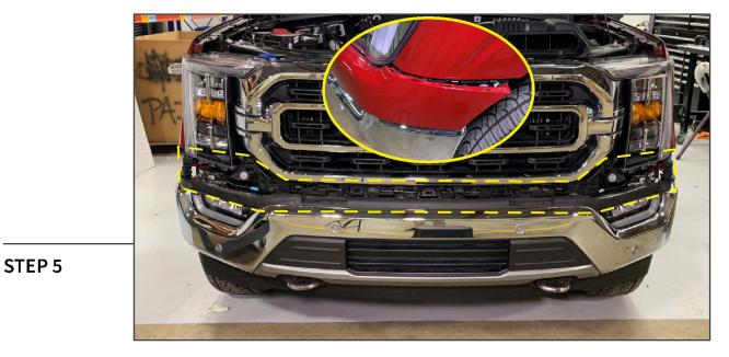
Pull the bumper trim away from the fender by firmly pulling the trim away. Repeat to the opposite side. Firmly pull the bumper trim from the vehicle and set aside.
