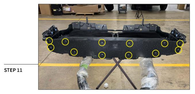
Route the grille emblem wiring/washer hose towards the top of the grille, if applicable. Plug in the included LED wiring harnesses, and neatly route upwards on the grille.
