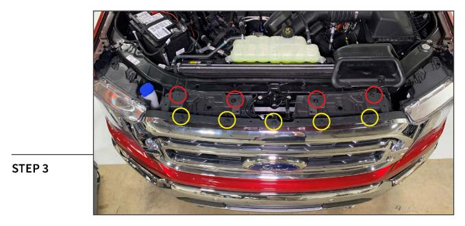
Remove (5) plastic push clips from the top of the grille. Remove (4) 10mm bolts from the radiator support to release the upper portion of the grille.
