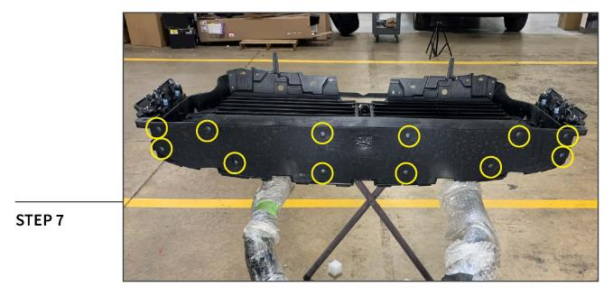
Remove (12) plastic clips from the lower portion of the grille. Remove the (4) plastic clips from each side splash shield. Remove the splash shields and set aside.
