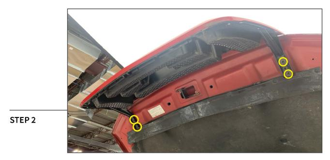
Remove (4) 10mm bolts connecting the grille assembly/brackets to the bottom of the hood. With the hardware removed, gently lower the vehicle hood to remove the grille from the vehicle.
