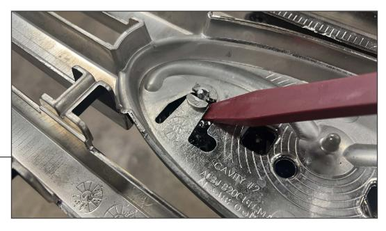
The grille emblem is double sided taped to the vehicle with posts fitted through the grille. Using a plastic pry tool, relieve tension from the posts while pulling/prying the emblem from the grille.
