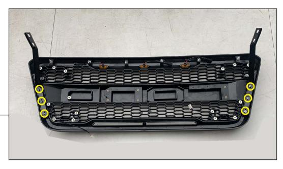
Place the new grille on a soft workable surface for assembly. Secure the LH and RH mounting brackets to the new grille using (3) Phillips screws and (3) flat washers per bracket.
