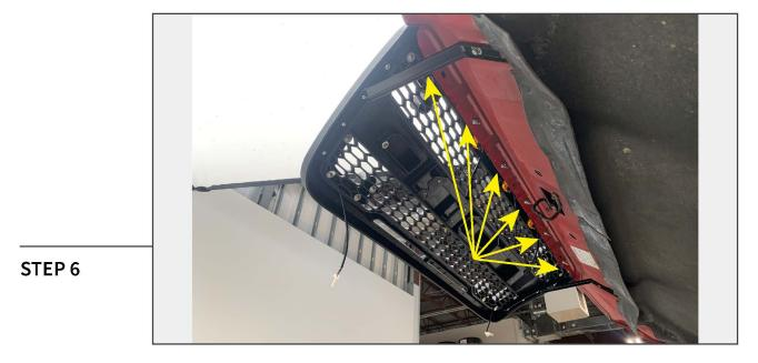
Align the grille to the vehicle, and secure the grille to the front of the hood using (6) M6 flange nuts.
