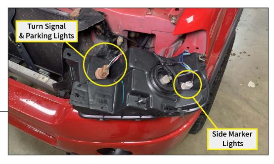
Remove the vehicle headlights by removing (3) 10mm bolts per light housing. Splice the DRL and turn signal lights to the vehicle headlight wiring following the diagram below.
